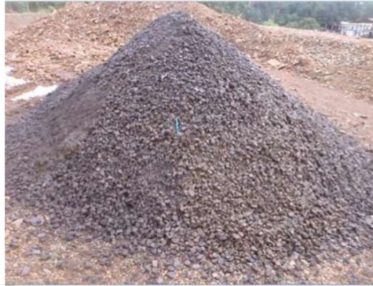
Figure 2 Nickel slag coarse aggregates after processing
